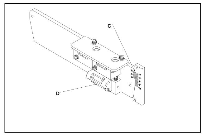
Figure 10 Aiming, Bubble Level & Vernier Scale
