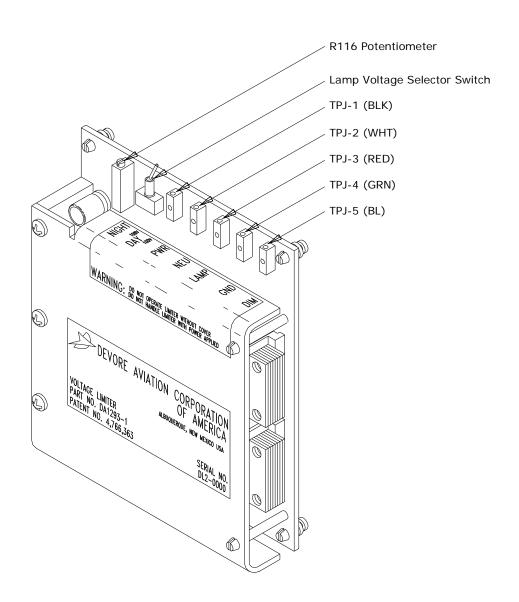
Figure 5a Voltage Limiter
