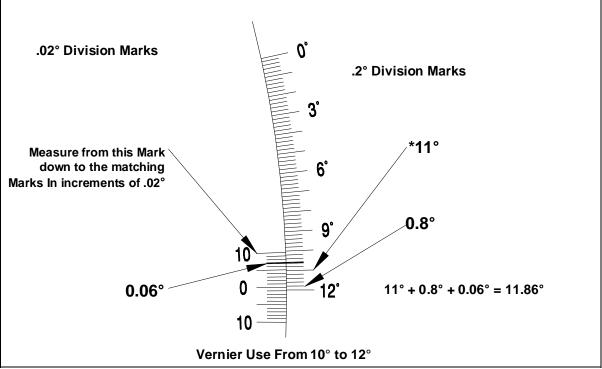
Figure 11 Aiming, Vernier Scale
