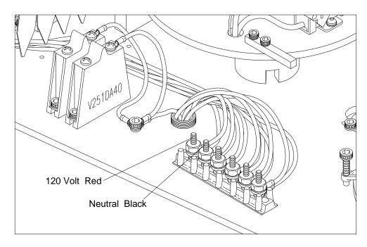
Figure 12 Voltage Test Positions
